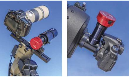
**SCOPING THE OPTIONS** Left: An Orion Mini 50mm guidescope and a ZWO ASI120MM-S guide camera are mounted in parallel on a dovetail bar with the imaging instrument, a Canon EF 300mm f/4L IS USM lens and an astro-modified Canon EOS 60D DSLR camera. Right: Both the guide camera and the imaging camera are attached to the telescope via an accessory off-axis guider. The device utilizes a small prism to direct part of the focal plane to the guiding camera.
