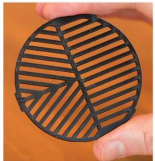
**DOING THE BAHTINOV** This sequence of images illustrates how to focus a lens fitted with a Bahtinov mask. When the central diffraction spike is positioned exactly halfway between the two diagonal spikes, the lens is perfectly focused. Left: This commercially produced Bahtinov mask made by Farpoint Astro installs much like a standard camera filter. The author uses it to focus his 300mm lens.
