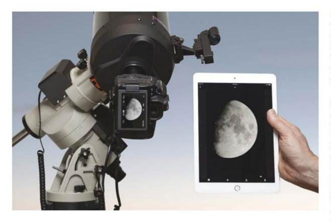
SIZE MATTERS The rear display of this Canon 80D is dwarfed by the iPad's 9.7-inch screen. Utilizing Live View on a large display makes obtaining perfect focus much easier, and because the connection is wireless, the display can be positioned at a convenient angle and far from the camera.
